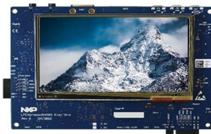
Fig 1. LPC54608 LPCXpresso development board
